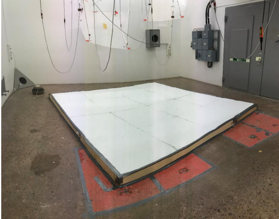
Picture 1 – Shows Spray-Tec-G with thickness 150 mm mounted on the floor in the reverberation room.
