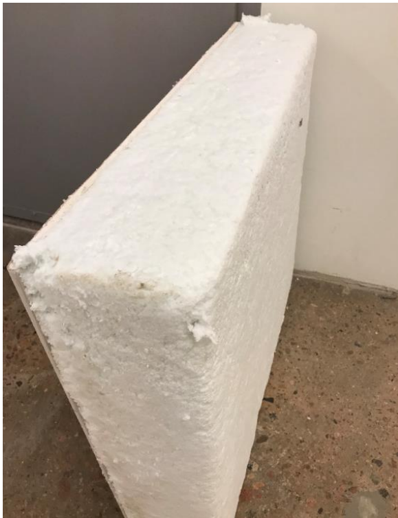
Picture 2 – Spray-Tec -G with thickness 200 mm.
